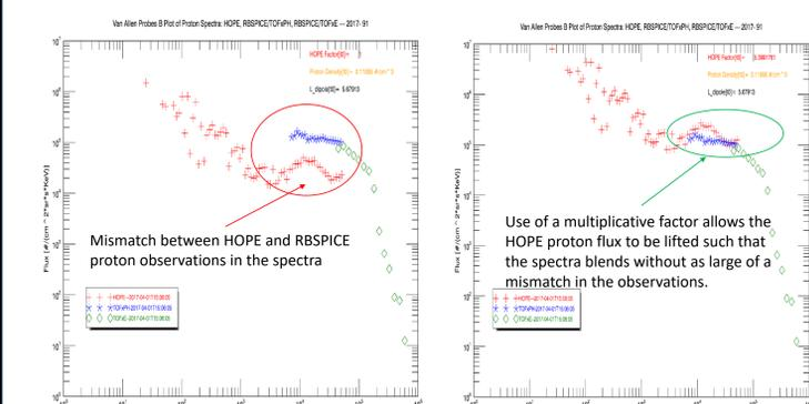
Algorithm to modify the Omni Flux from HOPE and RBSPI so spectrum are "aligned"
